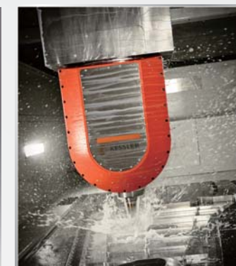
Multiple choose of 2 axis milling head and spindle HSK-A63 24000rpm & HSK-A100 12000rpm
